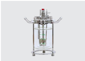
Mini Glass Vessel Water Jacketed Heating
